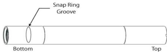
**C.** Coat Piston (12) liberally with rock oil - 200 centistroke and insert into bottom so Cylinder (10). Ensure it faces the right way as illustrated.
