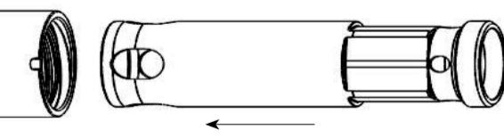
**I.** Fit 'O'Ring (9) onto Air Distributor (8). Insert Air Distributor (8) into Cylinder (10). Ensure it sits fully up against the Liner (11).
